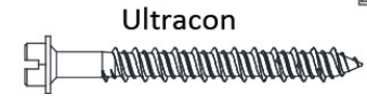
Ultracon ø5/16 HEX WASHER HEAD (HWH) 2 3/4" Minimum Length (For 1/2" max. shim space)
