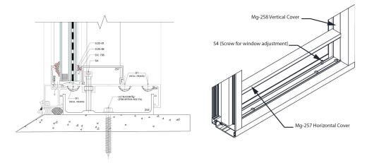
D. Via S4 screws at sill, adjust the level/height of the window. Adjust the
